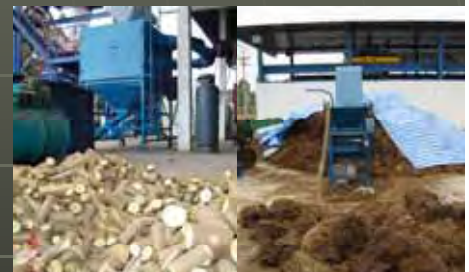
Small-scale Biomass Gasification Power Plant (Capacity 100 kw)
