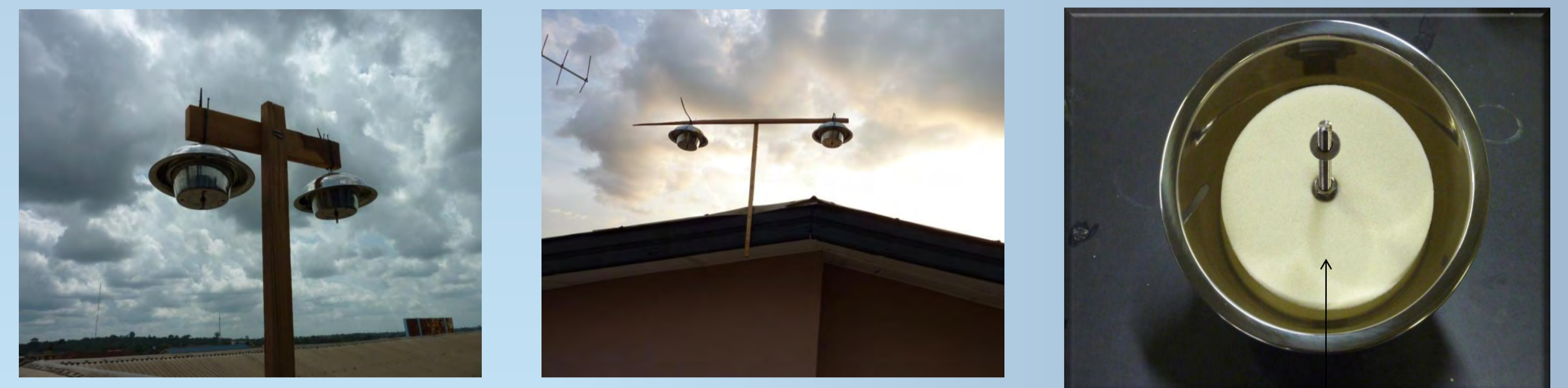
Fig. 1. PUF-disk PAS as mounted in the field in Ghana
