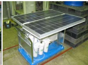
Installation of small solar-powered desalinization machine (PVRO)
